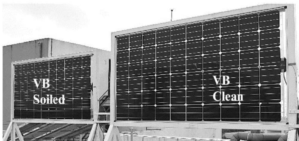
Figure 6: Vertical mounted bifacial PV modules (left soiled, right clean)
