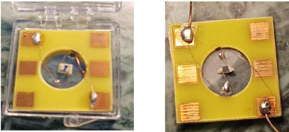
Fig:11: Device images of Hybrid Photodetector
