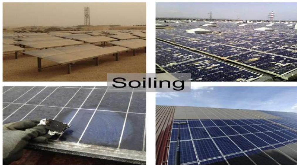
Figure 4: Soiling on PV modules [6]
