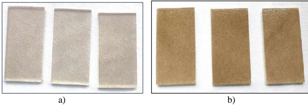
Figure 31: a) 0.2mg/cm<sup>2</sup>, b) 0.6mg/cm<sup>2</sup> dust deposition on glass samples
